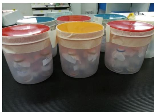
Figure 3.10 Fumigant toxicity test of powders of tested plants against adults of S. oryzae or R. domonica by vapour toxicity method
